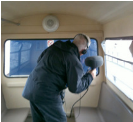
Kew Bridge Steam Museum Making an accelerometer recording of the Grand Junction 90” Engine. Image: RW
